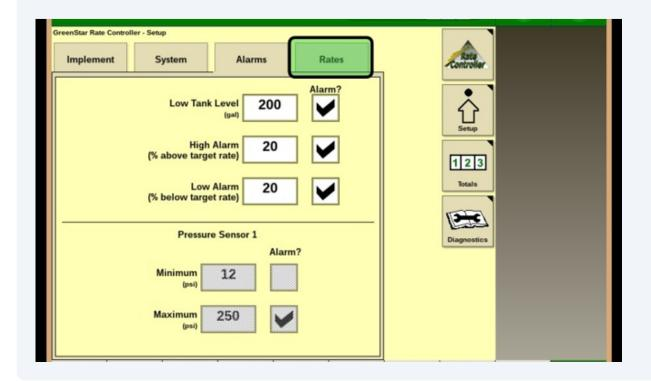
Operator should enter 3 preset rates to allow for easy switching back and forth on the main Rate Controller page. Once rates have been entered, switch the drop-down menu on the main Rate Controller page to "Predefined"
