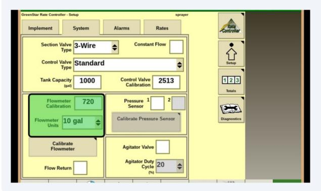
Pressure sensor & agitator valve boxes in Step 8 only need to be checked if they are wired into the Rate Controller system. If it is a manual pressure sensor, box does not need to be checked.
