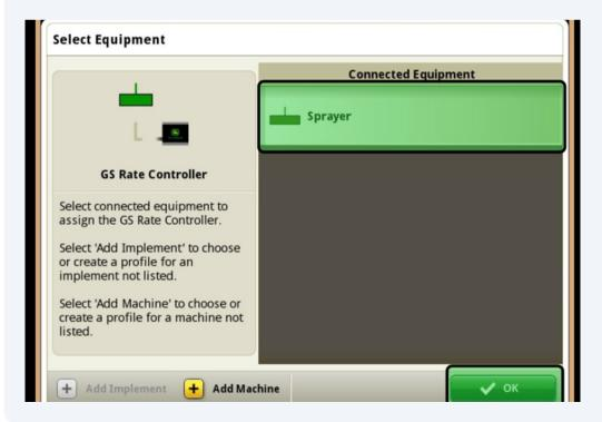
Verify Settings for the Implement Profile. This includes the equipment it is connected to, the working width, the work point measurement (Section Control runs off this measurement), and the mechanical delay on/off times. Once verified, hit Save
