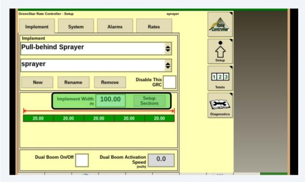
Tip! Up to 10 sections if there are no fence nozzles, Up to 8 with fence nozzles selected.
