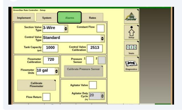
10 Check the boxes for each Alarm the operator would like to receive. Operator can modify each box to match their preferences
