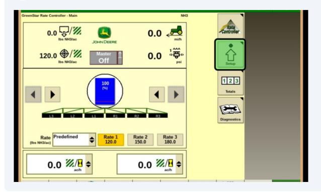
Select the correct Implement from the drop down. Select "New" underneath the bottom drop down and name your Implement. It's encouraged to be specific if the Rate Controller will be used on other implements in addition to the sprayer. Ex. "FAST 9600 Pull Behind" rather than just "pull behind sprayer."
